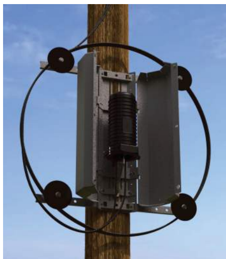
COYOTE 6.5" x 17" Dome Closure Mounted in COYOTE Defender with Dual Crossarm Adjustable Spool Vertical SLACKLOOP System
